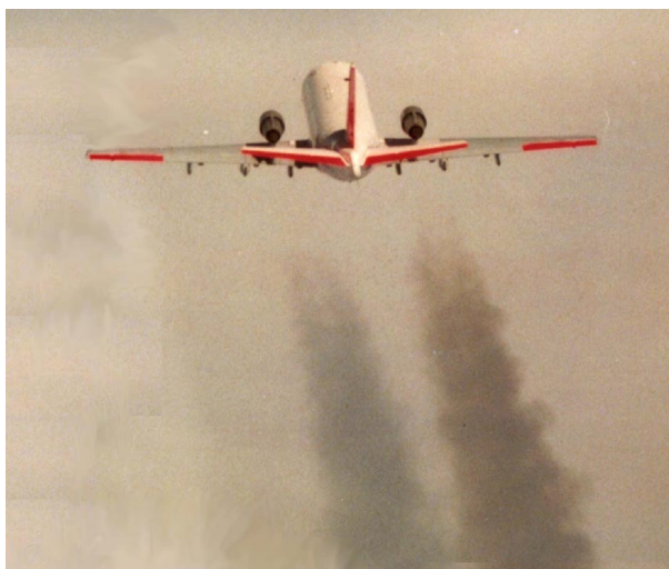
Figure 4.1: The ATTAS contrails seen from the Falcon aircraft at \sim 100 m distance. They form within about one wingspan behind the aircraft, in this case 25–35 m behind the engines. The sulphur (S) content was 170 (5500) ppm in the left (right) engine [Schumann et al., 1996]. The right-hand contrail becomes visible slightly earlier than the left one. In a similar experiment using fuel with 2 ppm and 260 ppm S, no visible difference in the contrails was detected [Busen and Schumann, 1995].
